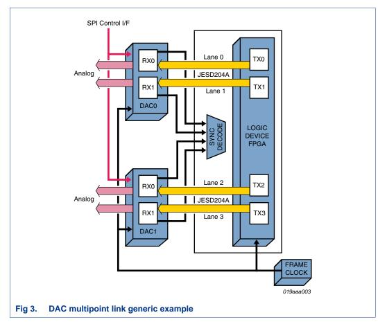
It is, in part, by virtue of the fact that there is a single frame clock and a single logical SYNC~ per JESD204A subsystem that sample time-alignment (and thus precise phase coherency) is possible among the data lanes.
