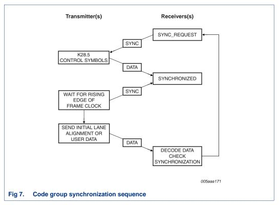
In systems with multiple lanes, the SYNC~ signals from all receivers (DACs or FPGA) are combined and asserted simultaneously to all transmitters (ADCs or FPGA). As long as a single receiver requests synchronization, all transmitters attached to the link or the multipoint link will send K28.5 control symbols during initial code group synchronization. The synchronization resolution is limited by the skew budget in the system.
