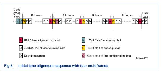
In the frame alignment monitoring protocol, 8b/10b user data symbols are used as periodic frame alignment symbols (a technique called character replacement) themselves, enabling frame alignment without data loss. There are two modes of this protocol, both of which use the K28.7 and the K28.3 control symbols.
