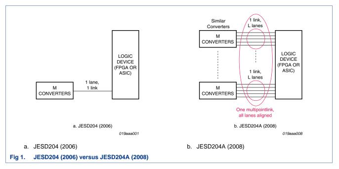
**Remark:** The scope of JEDEC JESD204A is constrained to the interactions between one logic device (FPGA or ASIC) and one or more converter devices (ADC or DAC).
